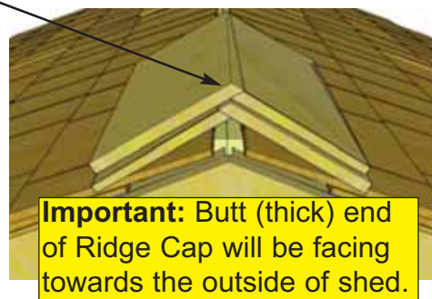
Alternate Ridge Cap seams (offsetting angle cut at peak)
